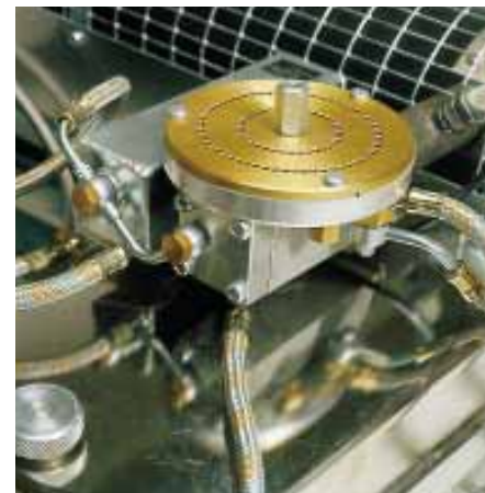
Air intake valve without filter acting as silencer.
